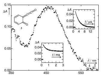
**Figure 3.** Spectrographic trace obtained by LFP of **1** in wet acetonitrile (10% water). The spectrum was recorded with a delay of 100 ns relative to the excitation pulse at 308 nm. The kinetic traces in the insets show the decay of transient absorbance at 450 nm in the same solvent mixture without (lower) and with (upper) addition of  $1 \times 10^{-3}$  M HClO<sub>4</sub>.
