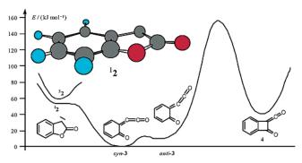
**Figure 1.** G3(MP2)//B3LYP zero-point energies (relative to *syn*-cumulenone **3**, Table 1) of the stationary points connecting 2-4. The structure shown on top is that calculated for the singlet carbene **2**.
