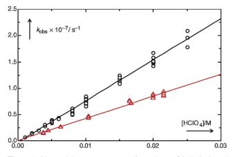
**Figure 4.** Observed decay rate constants of cumulenone **3** in H<sub>2</sub>O ( $\bigcirc$ ) and D<sub>2</sub>O ( $\triangle$ ) solutions at 25 °C as a function of perchloric acid concentration (data in Table S1).<sup>11</sup>
