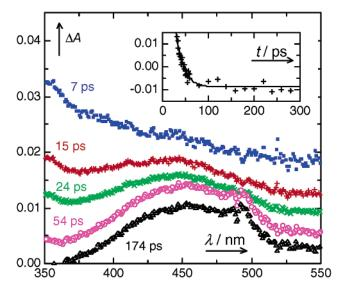
**Figure 2.** Picosecond pump-probe spectra of **1** in hexane. The kinks around 496 nm are artifacts due to the probe laser beam. The inset shows the loading coefficients of the second eigenvector determined by component analysis of 38 pump-probe spectra and a monoexponential fit function.
