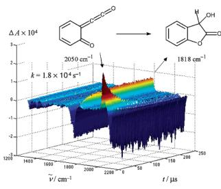
*Figure 5.* Temporal evolution of the IR difference spectra of 1 in CD<sub>3</sub>CN with 10% (by vol.)  $D_2O$  and  $1.0 \times 10^{-4}$  M DClO<sub>4</sub> after excitation at 266 nm. The concentration of DClO<sub>4</sub> refers to the total volume.
