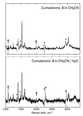
*Figure 6.* Transient resonance Raman spectra obtained for cumulenone **3** in acetonitrile (top) and water/acetonitrile (bottom) solvents. The numbers label the Raman shifts (in  $\text{cm}^{-1}$ ) of the resonance Raman bands of **3**. The asterisks mark solvent/parent band subtraction artifacts and the daggers represent ambient/stray light features.
